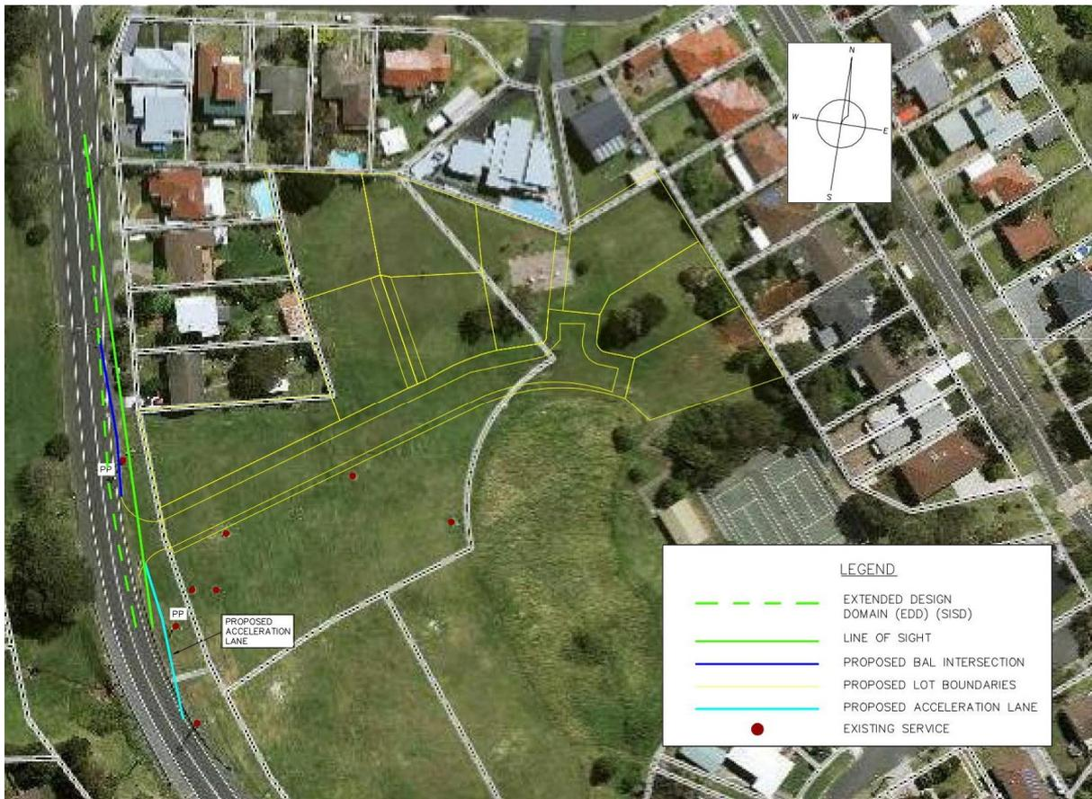
**Figure A2: Required Extend Design Domain Safe Sight Distance (EDD SISD) for proposed intersection**
