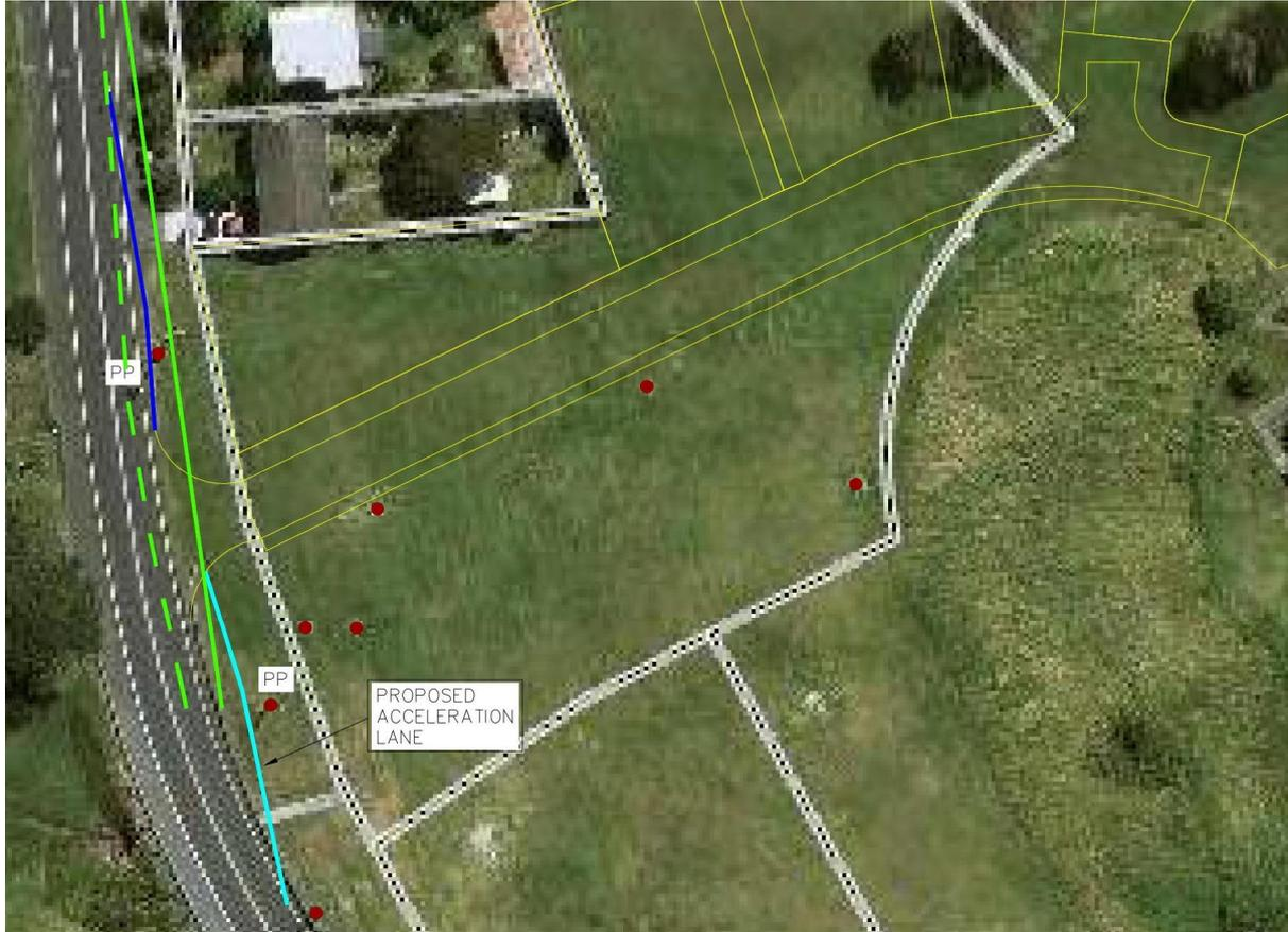
**Figure B1: Proposed BAL Intersection Overlay**
